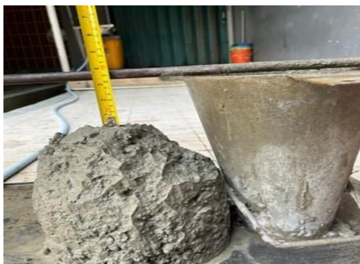
Slump Test Results for Concrete Test Specimens Variation 2
