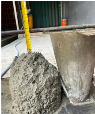
Figure 3. Slump Test Results for Concrete Test Specimen Variation 2
