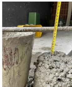
Figure 2. Results of Normal Concrete Slump Analysis Test
