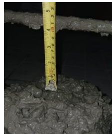
Figure 3. Results of Slump Analysis Test of Test Object Variation 1
