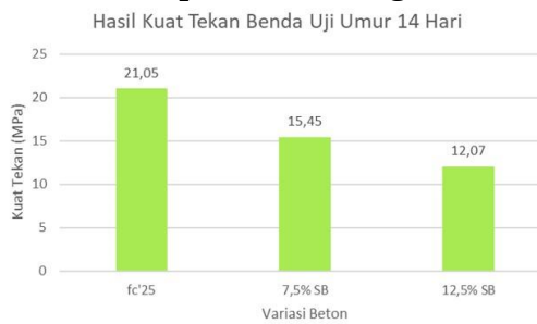
Figure 7. Diagram of Research Results on Concrete Compressive Strength at 14 Days
