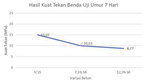
Figure 6. Graph of Concrete Compressive Strength Test Results at 7 Days of Age
