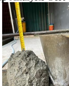
Figure 4. Results of Slump Analysis Test of Test Object Variation 2
