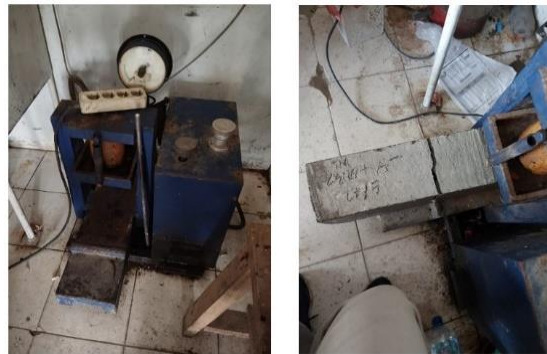
Figure 4. Beam Flexural Strength Testing Process
