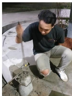
Figure 3. Slump Test Making Process
