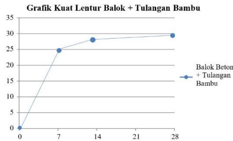
Figure 5. Graph of Flexural Strength Test Results of Beam + Bamboo Reinforcement Table 9 Summary of Flexural Strength Test Results of Beam + Bagasse Reinforcement
