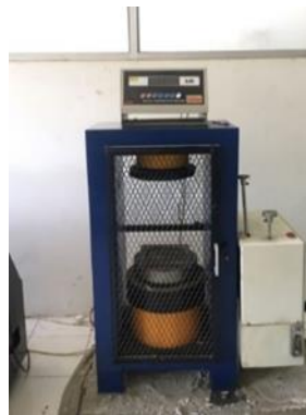
Figure 3. Concrete Load Compressive Strength Test Equipment
