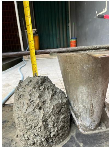
Figure 4. Normal Concrete Slump Test
