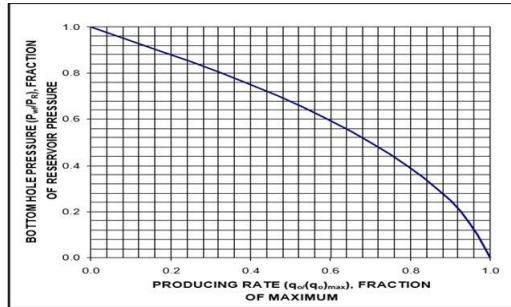
Figure 2. Two-phase flow IPR graph (Source: Pamungkasjoko,2010)
