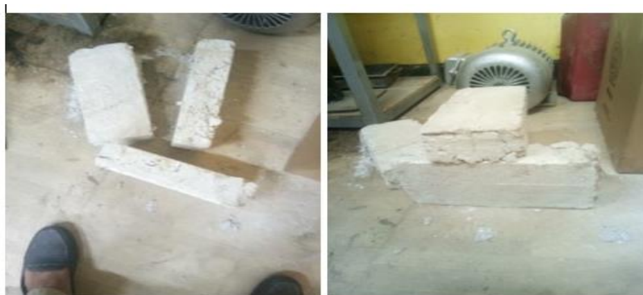
Figure 6: BTPSSK1 and BTPSSK2 which only had cracks after the compressive strength test
