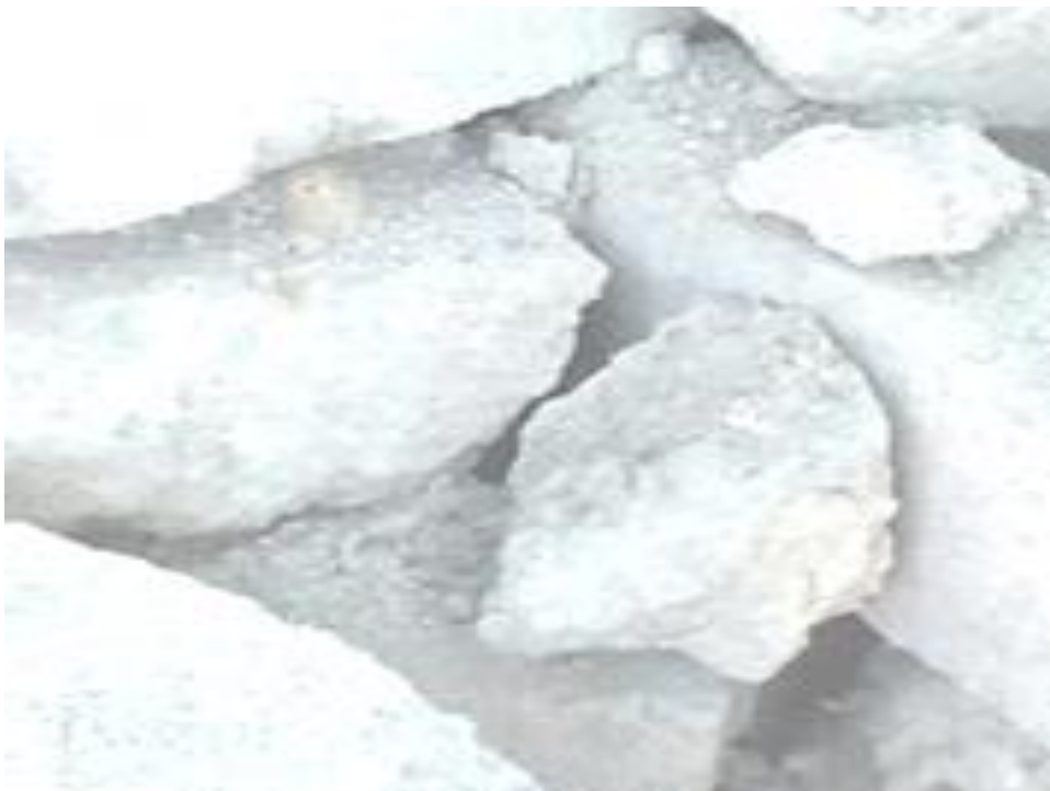
Figure 5: BTPSSK0 after being tested for compressive strength. Looks broken
